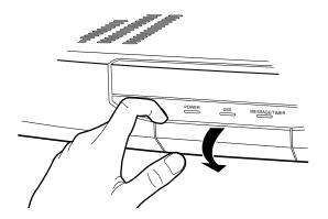
Then insert the card, arrow side up, as shown, and gently push the door up to close it.
